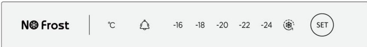
Temperature can be adjusted by pressing the 'SET' key. Every time when the "SET" key is pressed, the current mode indicator lights off while the next mode indicator lights up, with the said mode setting validated if no key operation within 5s (or else, the mode setting will be invalid). After the setting takes effect, temperature will be immediately controlled as per the mode setting.
