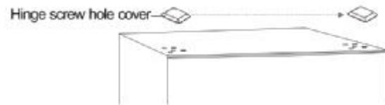
12. Secure the upper hinge to the top left side of the cabinet with the three screws you removed previously. Before you tighten the upper hinge screws, make sure that the top of the door is level with the cabinet and that the rubber gasket makes a good seal.
