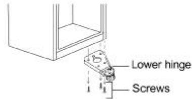
5. Remove the washer and nut that secure the pin shaft to the right hole on the lower hinge, then remove the shaft
