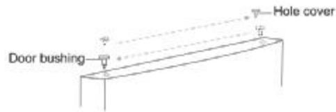
11. Remove the hole cover from the top left side of the cabinet and secure the cover on the top right side of the cabinet.
