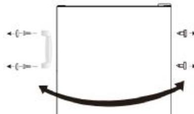
14. Install the right hole plugs on the left side of the door, and install the handle on the right side of the door.
