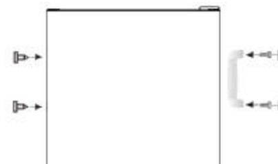
Note: Ensure the rubber gaskets are making a good seal with the cabinet all the way around the doors before tightening the hinge screws.
